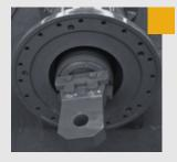
To prevent the terminal joint not to be cracking, reinforcment ring for each termal joint is added. For the guiding sleeve, we added two baffle rings with one swivel ring, to keep the kelly bar in staightness when it is under the state of force.
